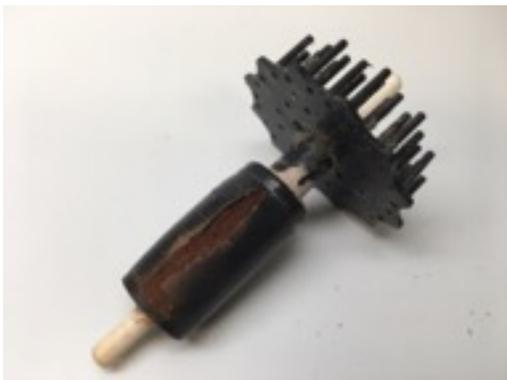
Split casing due to excess heat as broken through to magnet. This rotor is not usable.
