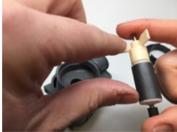
This Rotor and pump below show obvious calcium build up and need to be cleaned.
