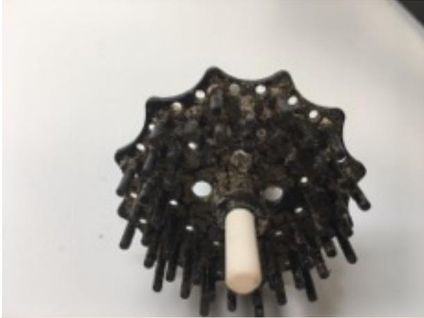
Dirty impeller needs Cleaning and can cause Noise, loss of flow or damage if rotor is out of balance because of debris.
