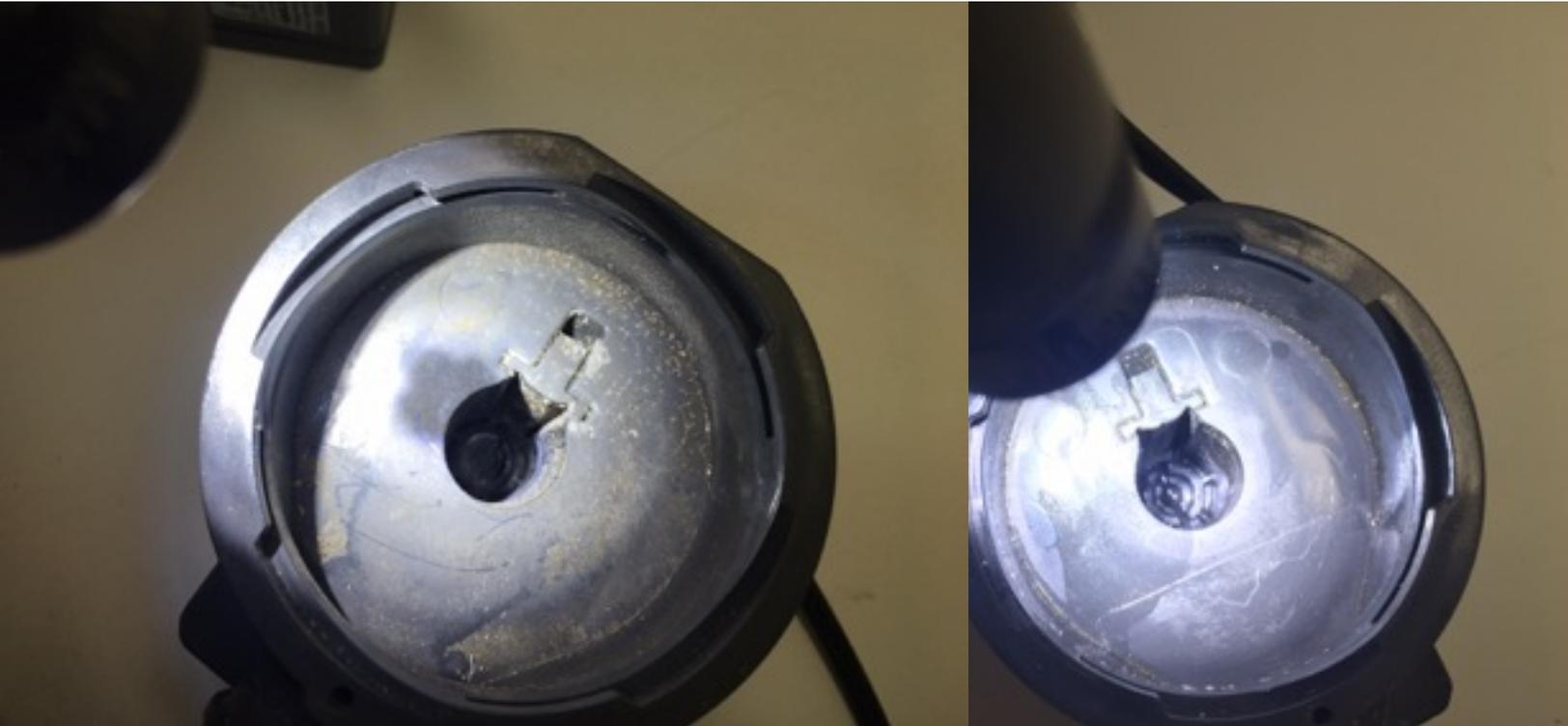
The Boot holders should be round and not worn larger or look melted. The upper left image has a boot holder cavity that are worn and will cause rotor movement, noise, and prevent proper function. The upper right image is a good
