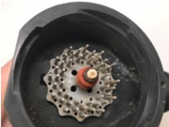
This red Rubber boot in the left image is worn and needs to be replaced. The bearings is also frozen due to calcification. In this case the strong pump turned the entire rubber boot inside its holder hole causing the damage. The pump has not been cleaned properly.
