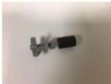
shaft separated from magnet. Although can be glued with super glue it is best to buy a new rotor.
