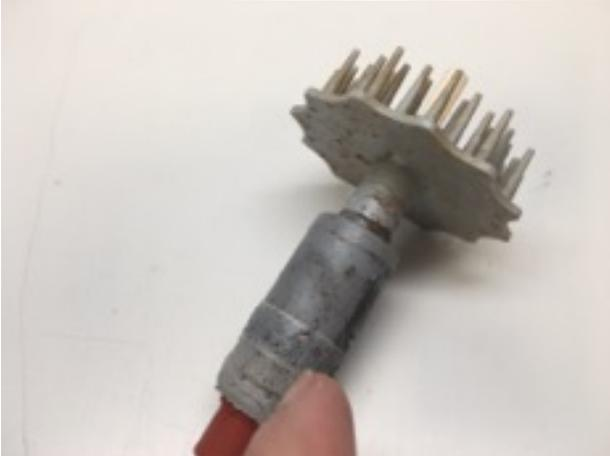
The Photo to the left shows burning of the rotor casing this is due to excess heat. Excess heat is caused from pumps running without enough water, or with frozen bearings.
