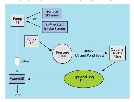
The diagram below shows a single pump installation.
